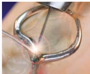
repair of broken clasp
