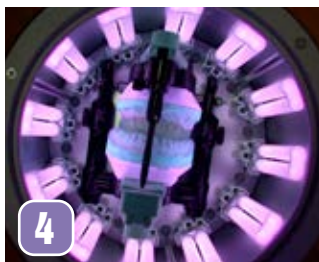
4 polymerisation in one of the metalight units...
