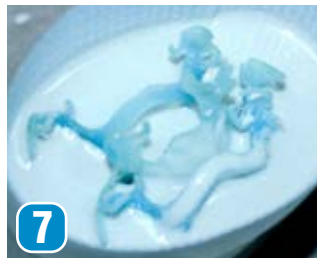
7 for best fitting the investment material expansion needs to be adjusted 10 % up
