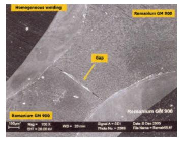
**Fig 13:** "Hollow seam" showing the internal gap, still as strong as a full material weld (picture courtesy of Prof. Lindemann, university of Tubingen, Germany)
