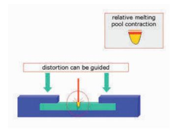
**Fig. 19:** The two objects are tightly secured so the melting pool cannot shrink toward the center but is "forced" to shrink downwards
