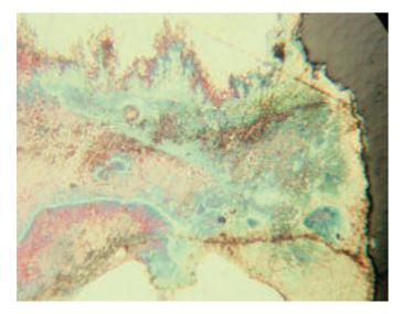
Fig. 3 Tarnished soldering^ metallographic cut, Hellfefd, 50  $\times$  magnification
