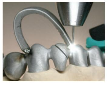
**Fig. 20:** The cast bar is connected with one or two pulses to each of the two parts to be joined. After welding, the bar can be easily removed by hand.
