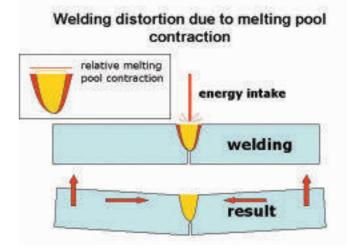
**Fig 18:** The yellow area shows the dimension of the welding spot in the solid stage, the red areas (left and right) show the expansion of the welding spot in the liquid stage.
