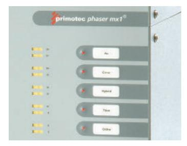
**Fig. 14:** Primotec phaser mxl preset programs for Gold, Cobalt-Chrome, Hybrid (Gold to Co-Cr), Titanium and orthodontics
