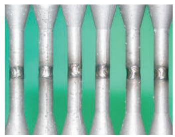
Fig. 9: specimen fully welded for standard testing
